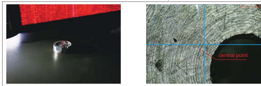
laser indicator locates the central point
